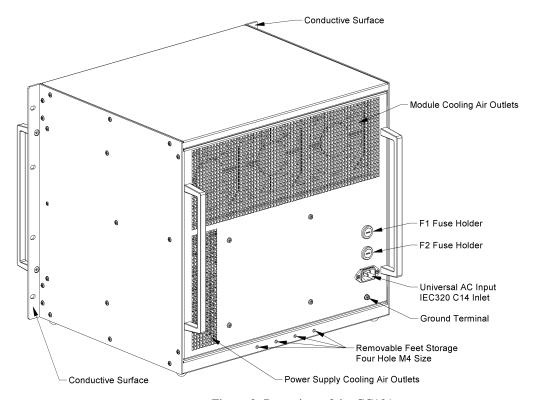
Figure 2: Rear view of the CC121
